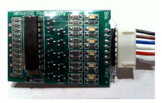
When the Blinky is first connected to the battery pack, the leftmost 4 red LEDs will stay on for 3 seconds. This indicates that each cell is at least 2.8 VDC, which is the minimum voltage to start charging with high current.
