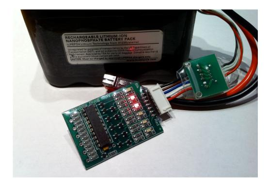
If no LEDs light for about 5 seconds, the cells are balanced.
