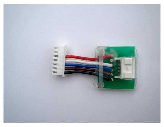
The Blinky is marked with Blk and Red on the corners on the end beside the protruding pins. It should be inserted into the socket so those markings match the color of the wires. As you can see in the photo below, the Blk corner is on the end of the white connector socket where the black wire is. Only 5 pins of the 7 pin socket are used. That's 1 for ground, and 1 at each positive battery terminal of the 4 in series.
